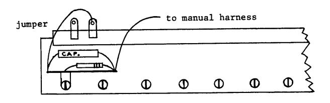
CAUTION: Remove only one bolt at a time. Replace and tighten each bolt before removing next one.
